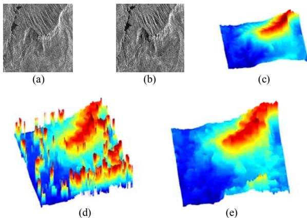
Fig.2. (a) and (b) : RADARSAT images in epipolar geometry . (c) : 3D view of the reference disparity map, (d) : Classical matching method, (e) : Coarse-to-fine method.
