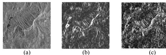
Fig.3. (a) SAR image, (b) ROEWA operator, (c) Deriche Operator
