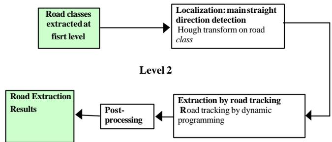
**Fig. 4.** The road extraction procedure
