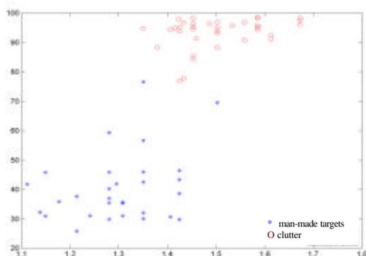
**Fig 7:** Fractal dimension versus energy in bright scatterers of natural clutters (circle marker) and man-made targets (asterisk marker).
