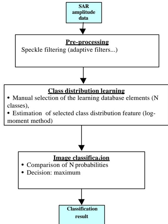
Fig. 2: Level 1; ML classification of filtered data.
