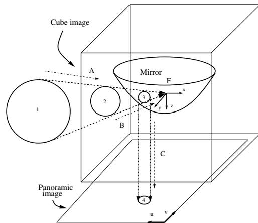
**Fig. 2.** Panoramic image synthesis principle. A: Projection from the scene to the cube faces. B: Projection from the cube faces to the mirror. C: Projection from the mirror to the panoramic image plane.
