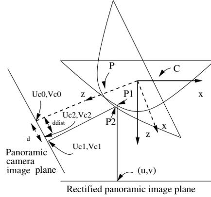
**Fig. 11.** Panoramic image rectification principle
