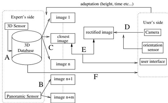
**Fig. 1.** system principle: A: 3D Acquisition of the site; B: Panoramic images acquisition and rectification; C: Synthesis of omnidirectional images; D: User's image rectification; E: Matching; F:Guidance
