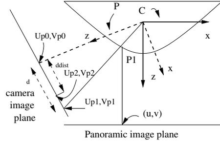
**Fig. 7.** Standard image rectification principle
